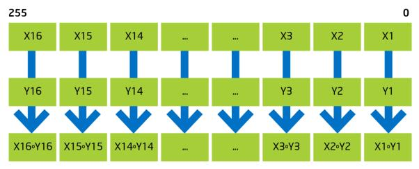
Figure 4: Processing data in parallel with Intel SIMD instructions
