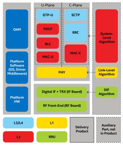
Figure 1: Evolved Node B(eNodeB) functionality example
